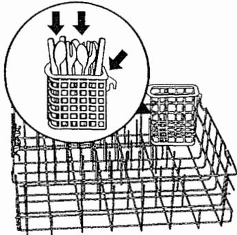
The utensil caddy has three hooks. (See arrows.) For best wash performance, hook the utensil caddy in the right rear corner of the lower rack. You can also hook it in the left front corner.
