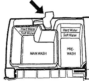
2. Add the correct amount of detergent to the Main Wash section of the dispenser according to the chart below. If you are using a tablet detergent, it must be placed in the Main Wash section. (See "How much detergent to use.")
