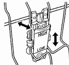
2. With the other hand, pull out the top of the adjuster.
